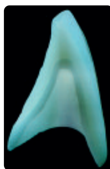
IPS e.max Ceram on ZrO 2 in transmitted light
